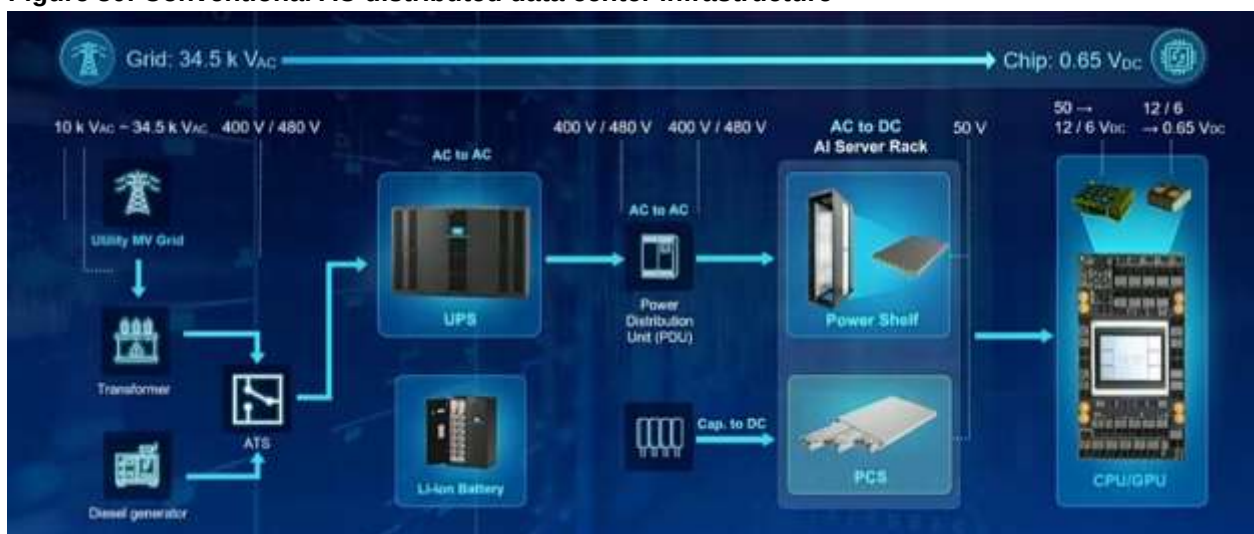
Figure 80: Conventional AC distributed data center infrastructure
