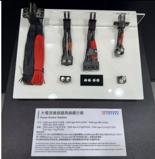
Figure 6: GB200 power busbar at HHTD 2024
