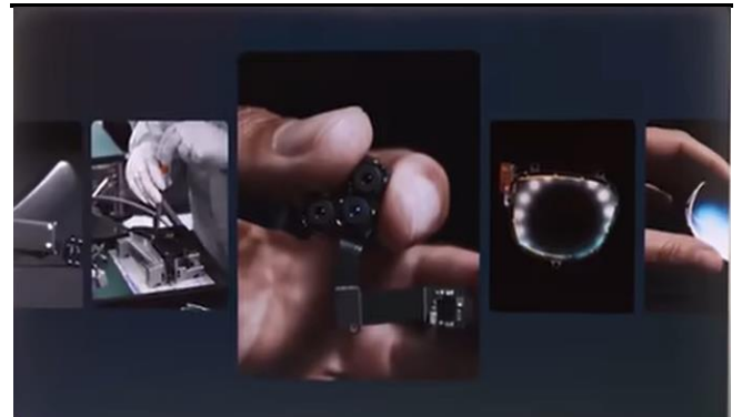
Figure 7: Meta Orion-projectors in glasses arms that shoot the lights into wave guides
