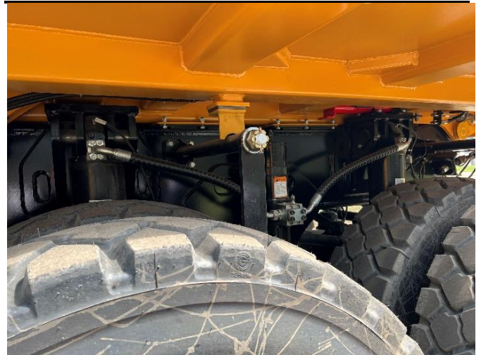
Figure 4: SANYI's 2nd generation wide body truck equipped with hydraulic cylinders to enhance shock absorption
