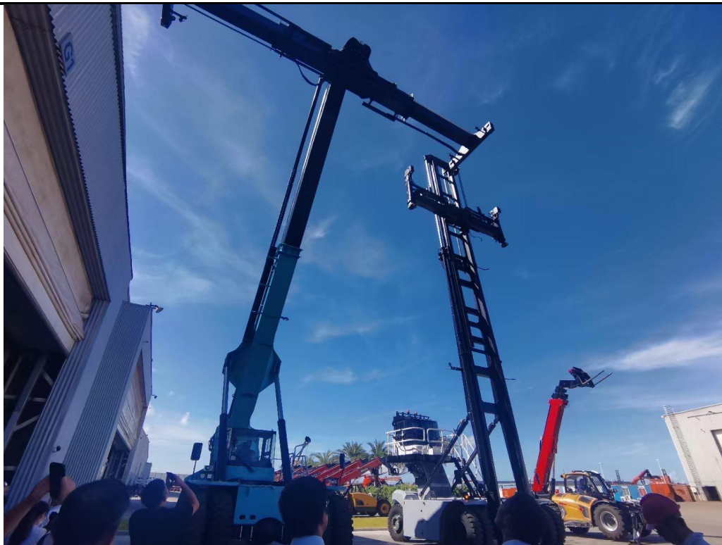
Figure 1: Electric reach stacker (left); Electric empty container handler (middle); Telescopic forklift (right) in Zhuhai production base
