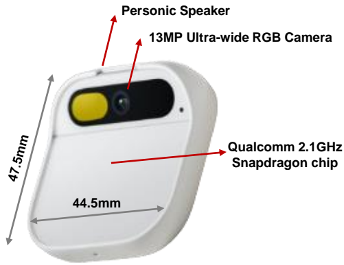
Figure 1: AI Pin specifications
