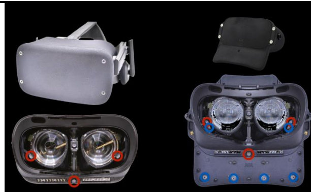
Fig.22: Meta’s headset cameras for gesture tracking
